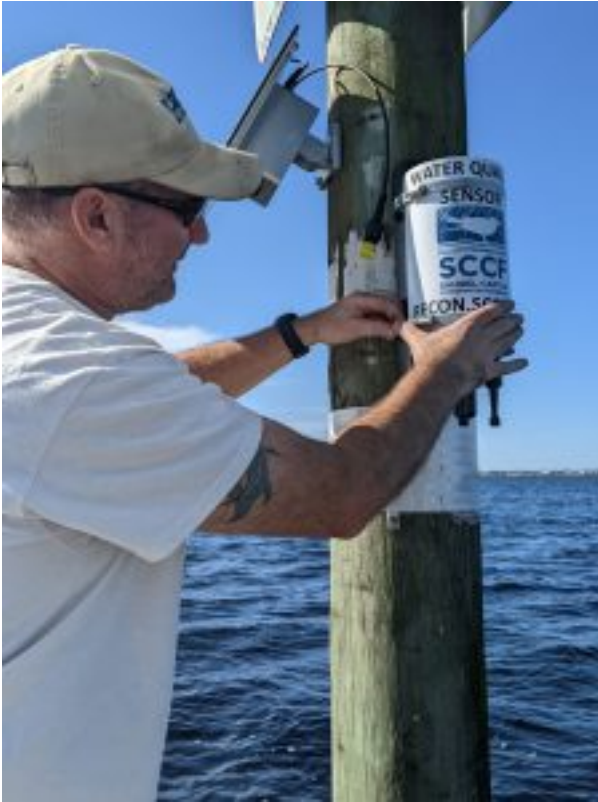
A.J. Martignette, with the Sanibel Captiva Conservation Foundation, installs a RECON water quality sensor. (Photo courtesy of Sierra Greene)
