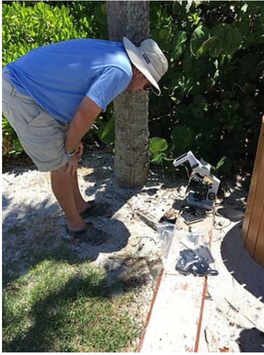
HABscope is a citizen science device used for water sampling. A 3D-printed attachment connects a smartphone device to a microscope to get close-up video images of microscopic organisms in water samples.
